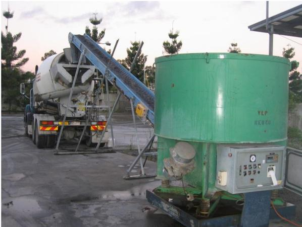
For this project, Fibercon are supplying Hanson Concrete with 1200kg Bulker bags, and the material is automatically dosed using a specialised dosing machine.
