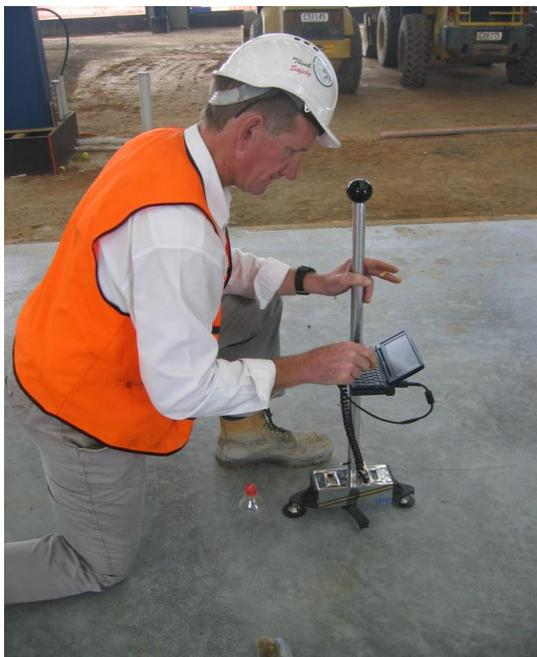
One of the benefits of using the Somero Screed and a fast placement system is that extremely good floor tolerances can be obtained. The first slab was less than 1mm in three metres deviation
