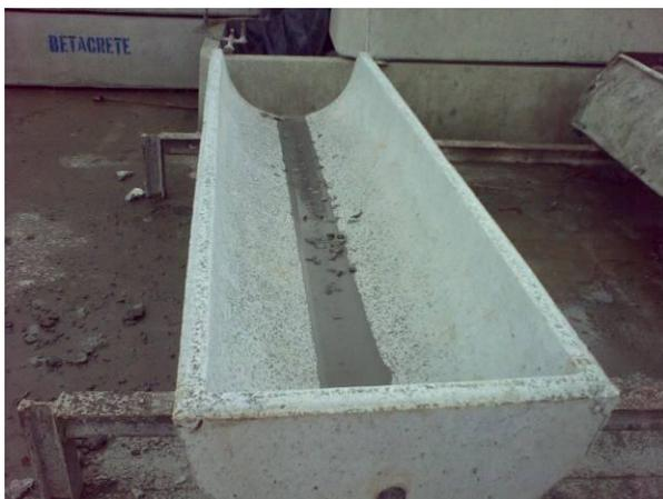
Fibercon steel fibres have been used for over 20 years in Septic and Water tanks, and are approved for Australian Standards AS1546 – Septic Tanks. Precasters are also having success in Pad Mounts, specialised pits and difficult shapes.
