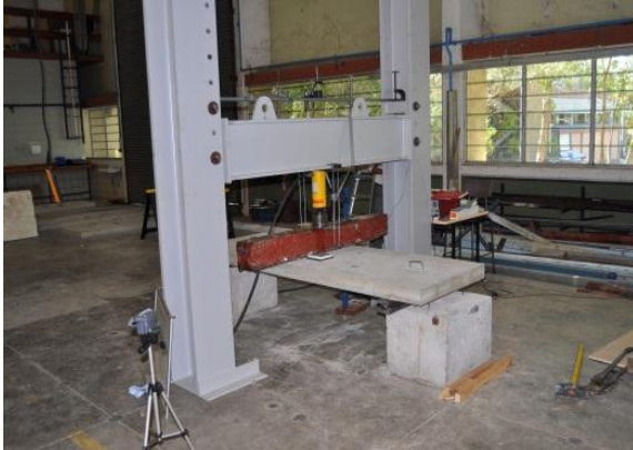
Testing of a one way slab with fibre and L Class Mesh
